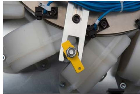
Incorrect: disk is not secured
